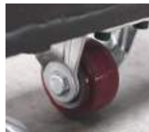
Two casters for quick repositioning of manipulator.
