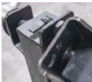
Three Locking Positions - 0° and 30° on both sides.
