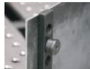
Magnet keeps sheet metal in vertical position
