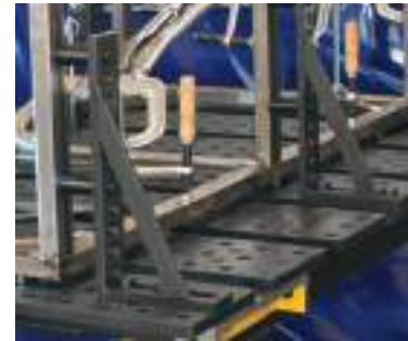
Insert V-Blocks to support round stock.
