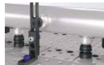
Vertical application using Locating Post + V-Block Spacer
